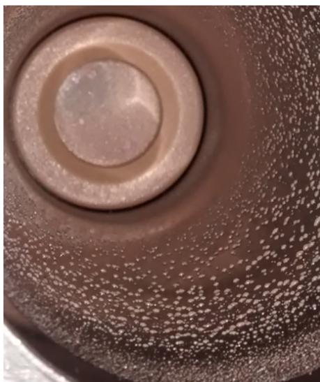
Fig. 3. Photography of the inner SAS precipitation cell after decompression.
